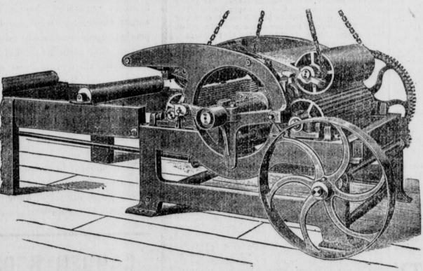
This machine has been designed to meet the requirements of all saw mills, whether for use in portable or stationery mills. The machine will take saws up to 20 inch diameter.
