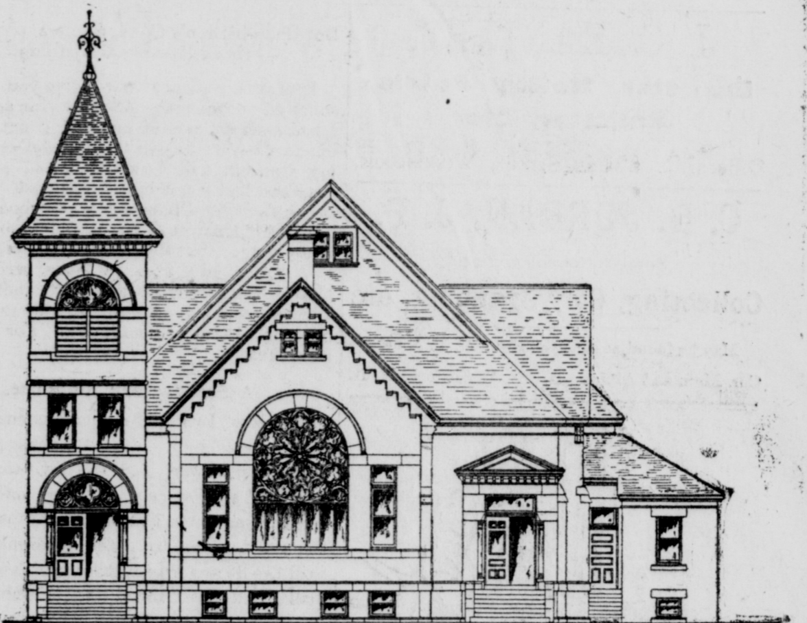
Chapel Street elevation of new Methodist Church, taken from the architect's drawings. The corner stone rests at the top of the steps at the extreme left or west corner. The length of the building on this street is 63 feet, not including the minister's room, which is not flush with the main elevation. The tower is 65 ft. high.
