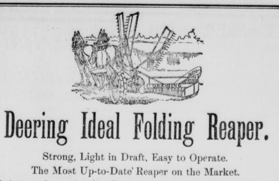
An important feature of the Ideal Reaper is the ease and dispatch with which the driver can make every adjusament to meet varying crop conditions without dismounting from the seat. He can quickly adjust the rakes to sweep the platform, to have them act as reels without sweeping, or tilt the platform to throw the knife down to pick up lodged grain.
