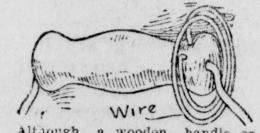
Although a wooden handle on title is supposed to protect the hand frequently happens that the handle sorbs enough heat from laying on the metal part of the kettle to cause never burns. Besides, it has fre quently happens that the handle is burned or charred. A good way to prevent both of these happenings and keep the handle cool is to attach a soil of wire to one side of it, as shown in the sketch. This keeps the bandle sway from the kettle, and while it may get warm will never get hot.
