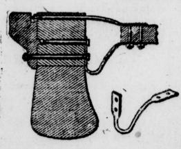
with this device does not extend into the head but is fastened to it by means of two short spring-steel rods. One of these is bolted to the upper edge of the wooden member and the other to the lower edge. The former extends through the head and is fastoned by a nut; the latter describes a downward curve and is fastened to the head by two bolts. This gives the head by two bolts. The head by two bolts. This gives the head by two bolts. The head by two bolts.
