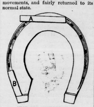
In the cut, A represents outside toe. B lengthwise heel calkin.
