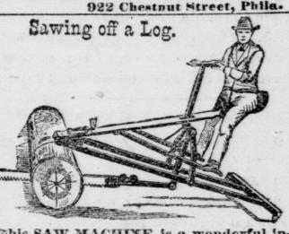
This SAW MACHINE is a wonderful invention. The weight of the man who is sawing does half of the work. It saws logs of any size, and will saw off a 2 foot log in 2 minutes. Circulars free. Address. Wm. GILES, 696 W. 6th St., Cincinnati, Ohio.
