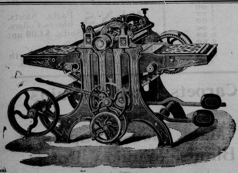
Revolving Bed Surface Planer. SPECIALLY ADAPTED FOR SURFACING GREEN, ICY, WET OR THICK LUMBER.
