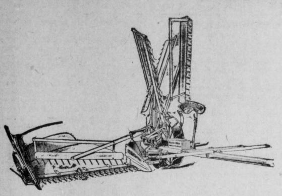
The main frame is cast in one piece and keeps all shafts and gears accurately aligned. The platform is joined to main frame by a strong hinge we I braced in every direction. The gearing is enclosed. Instantly adjustable as to height of cut and tilt of guards. One or more or all of the rakes can be made to rake or to act as beaters only.
