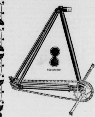
This Cycle has more improveme ts (not changes) of merit and importance than all others, amongst which are its Patent Oil Bath Bearings, Locked Adjustments, Patent Reversible Seat Pillar, the neatest and most effective adjustable Handlebars, correct Chain Alignment, Narrow Tread, with absosolute Rigidity, Double Rear Crown
