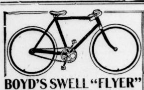
1900 MODEL. New ideas, new design, 11/8in. tubing, flush joints, Springfield one-piece cranks, high grade in every detail. Fitted with Victor tires, \$35.00; with Morgan & Wright tires, \$37.50; with Dunlop tires, \$40.00. Men's, 22 and 24 inch; Ladies', 20 and 22 inch frames. Black and maroon
