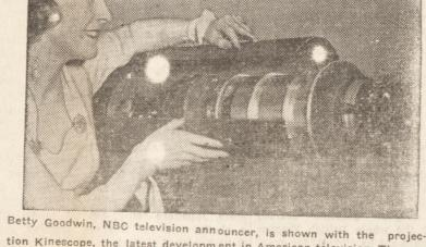
tion Kinescope, the latest development in American television. The new Kinescope throws an image three f eet by four feet on a picture screen.
