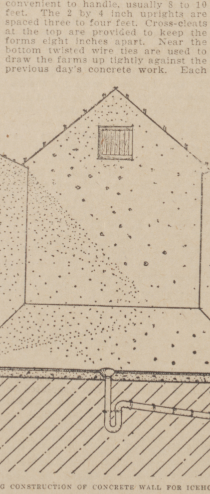
SHOWING CONSTRUCTION OF CONCRETE WALL FOR ICEHOUSE.
