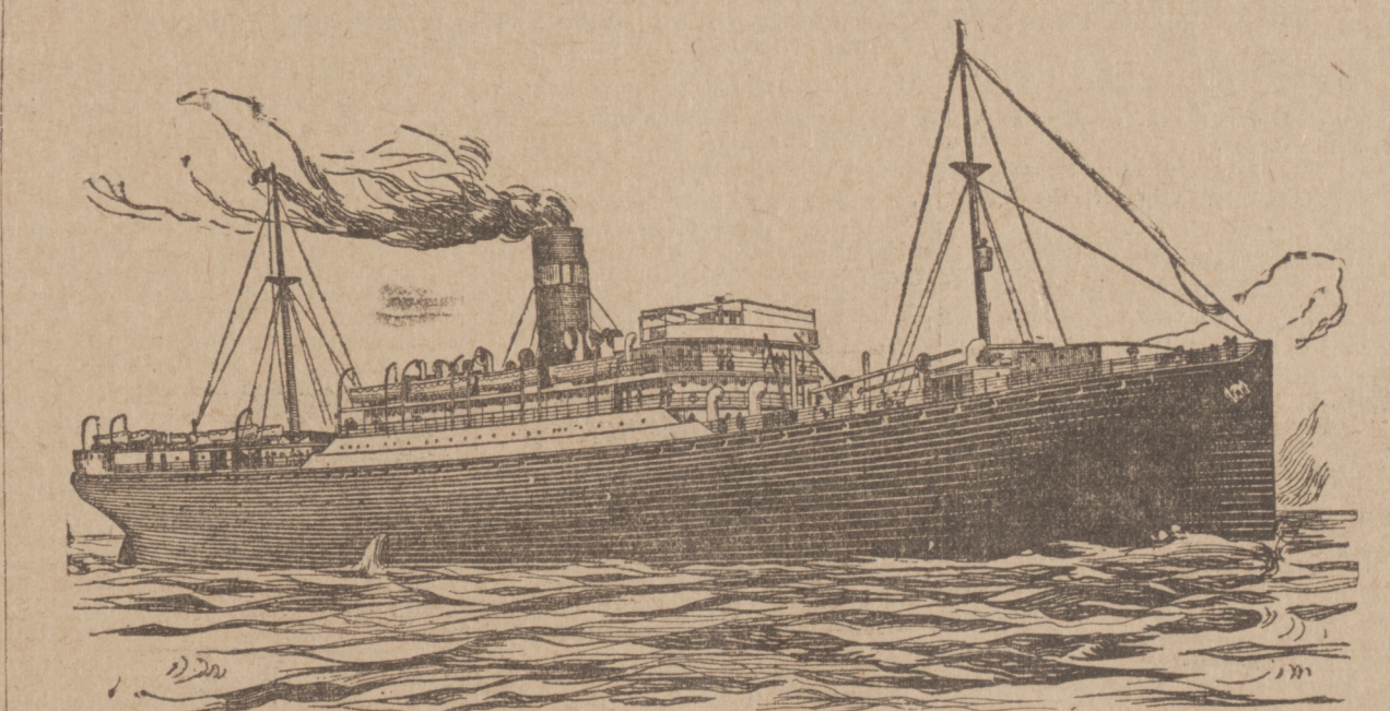
Length, 445 feet; breadth, 53 feet; depth, 33 feet; net tonnage, 4,726; gross tonnage, 7,396 tons. She was built in 1906, at Greenock.
